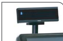
PD-2501 11 mm x 20 VFD display, 5X7 dot matrix, RS232 interface.
